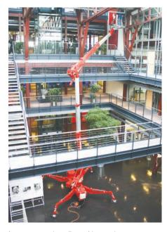
Its compact size allowed it to gain access through the narrow doorway. This particular Spider proves popular due to its variable jacking and large 11.20m outreach, allowing workers to set the machine up in small, enclosed places.
