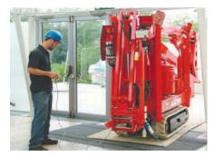
Non-marking tracks were suitable to use on the recently laid tile floor.
